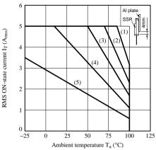
Fig.3 RMS ON-state Current vs. Case Temperature
